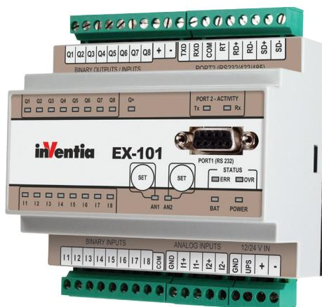
The EX-101 is an extension module for MT family of telemetry modules. It is optimized for use in advanced measurement systems equipped with 12/24V power source. Additionally, it can act as a universal I/O station with galvanically isolated RS232/485/422 Modbus RTU interface. The ability to run local control program allows to use EX-101 module as freely programmable PLC.
